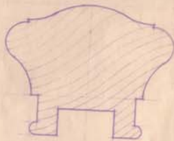
HANDRAIL (QUALITY) BILL COON
